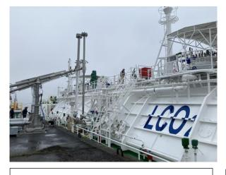
$\cdot$  "EXCOOL" berthing at onshore terminal Liquefied CO2 is being transferred through the loading arm shown in the middle.
